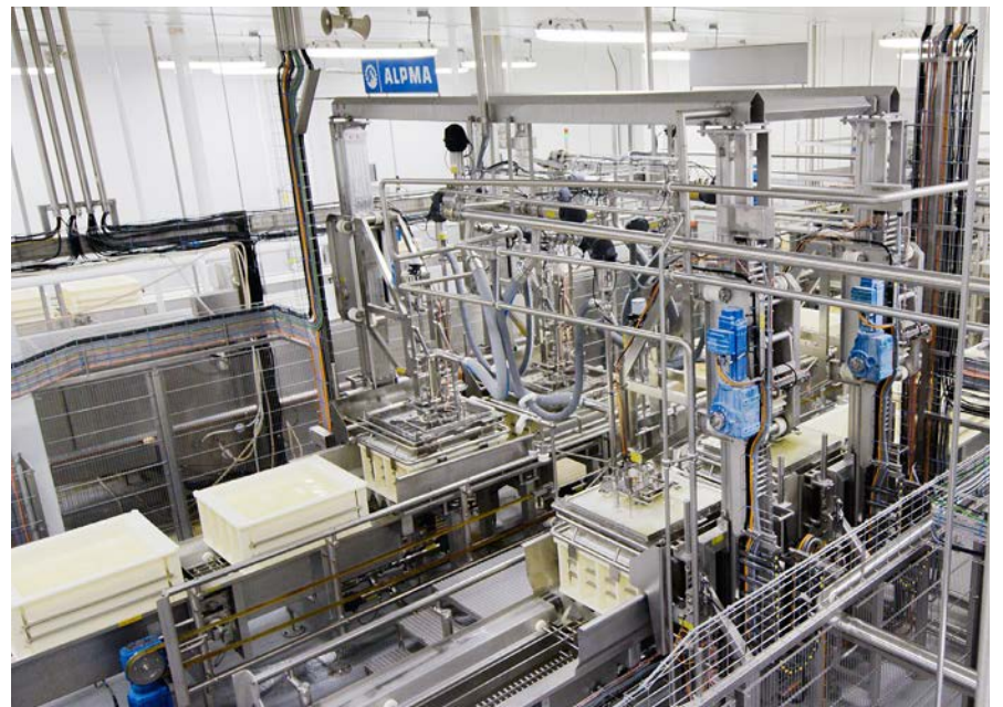
Luana’s latest expansions include a new process room. The Alpma system fills the 200-pound cheese moulds with curd, presses the block, cures, and then de-moulds the cheese before hitting the brine.
