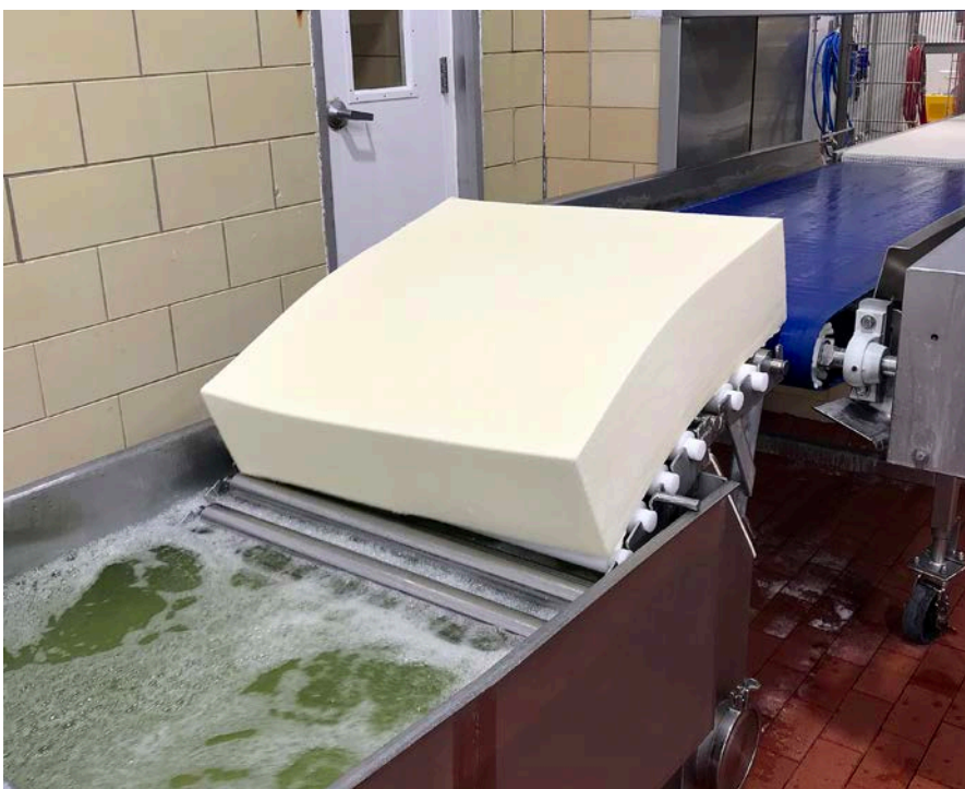
A 200-pound Swiss cheese block exits the block forming and filling room, and enters the brine flume at Prairie Farms' Luana, IA, plant
