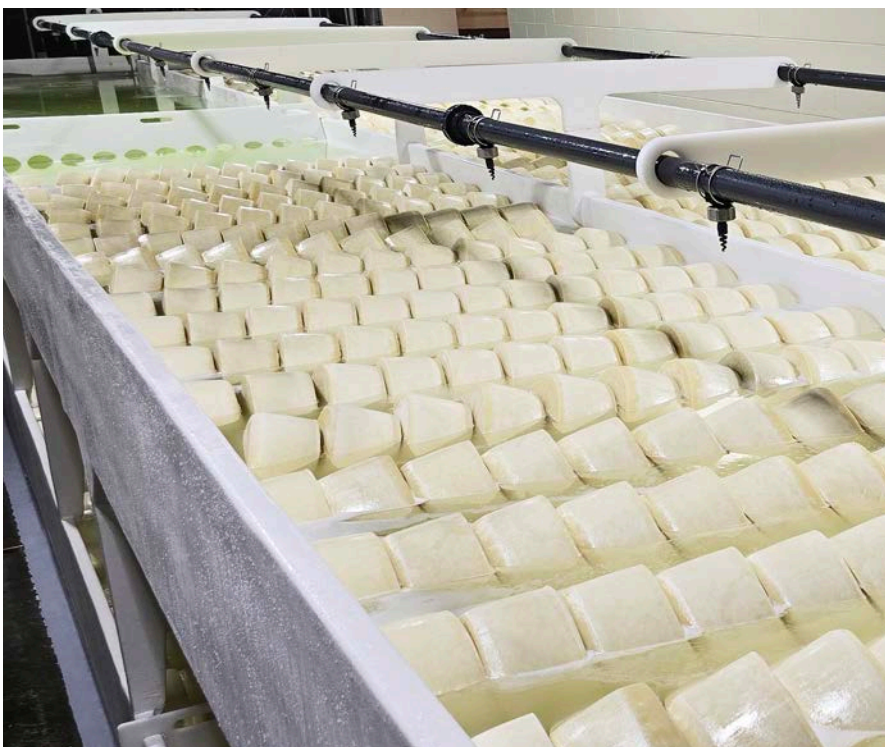
Eau Galle Cheese makes 20-pound wheels of Parmesan cheese which are brined in tanks made by Fiberglass Solutions, Inc.
