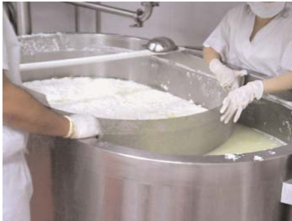
At the South Texas Artisan Cheese Company in Edinburg, TX, operators need to import milk all the way from Wisconsin due to an inadequate milk supply. In the above photo, cheese makers drain the whey from a vat of hispanic cheese.
