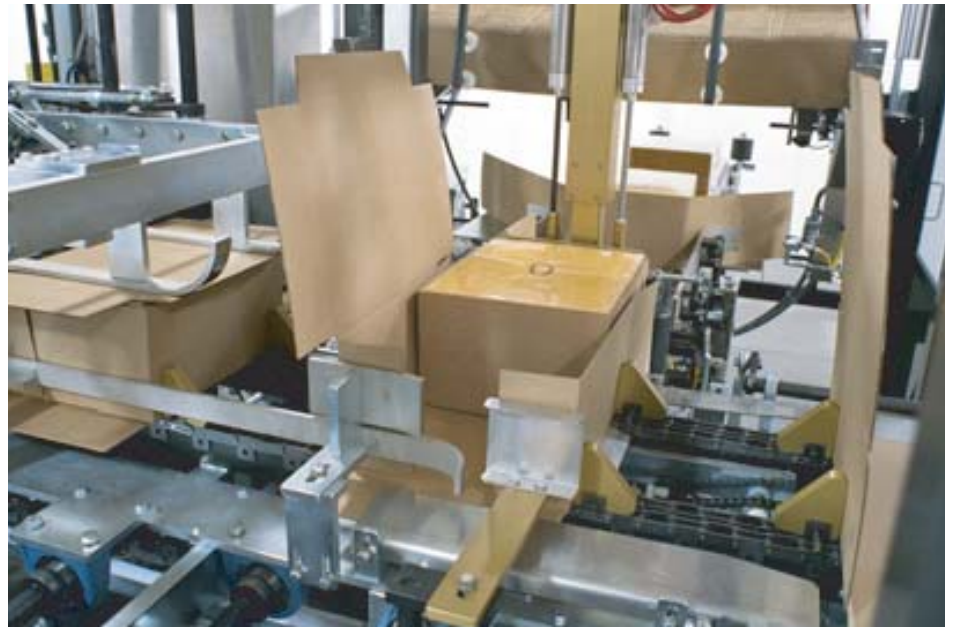
Mullins Cheese recently put into two Massman case packers into its two cheese operations. The application pictured above has the cheese block being moved into the wraparound case after the collar is placed and formed. The case packer can load 25 40-pound blocks a minute.
