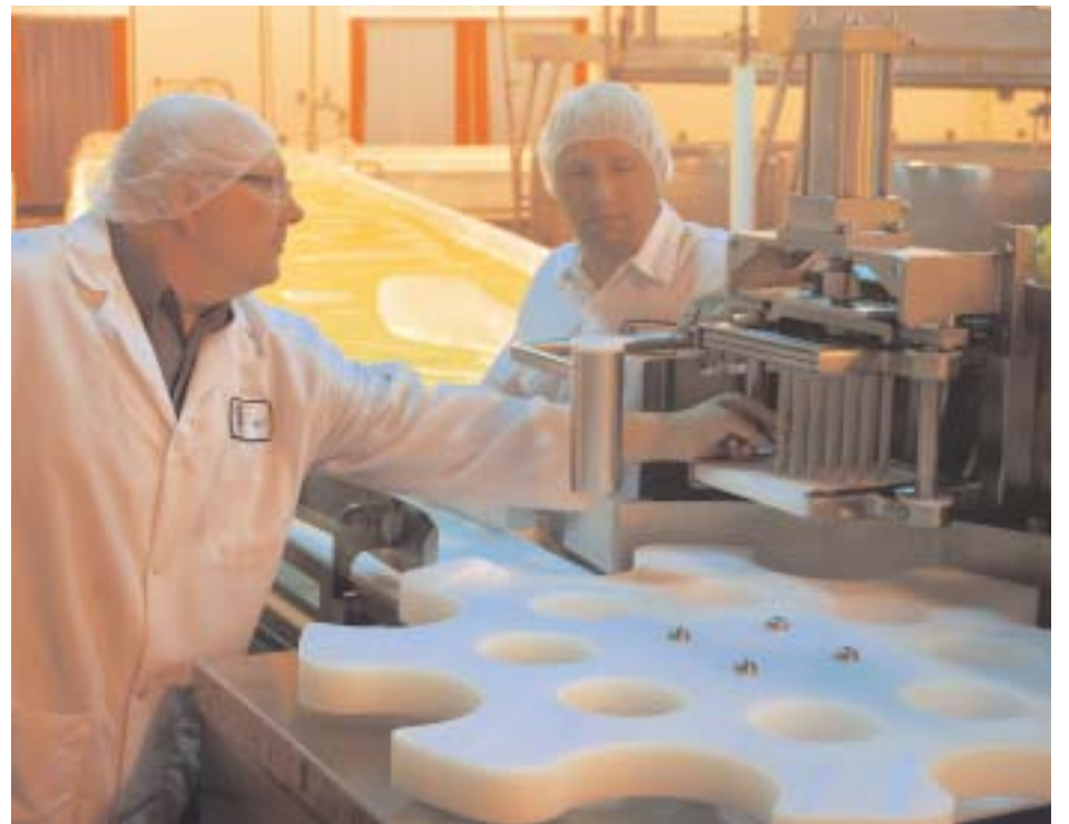
Mike Brennenstuhl and Rob Richter of Seymour Dairy prepare their new Johnson Industries Blue cheese piercer for production. The cheese piercer has put an end to the bottleneck area of piercing and handling the blue cheese, Brennenstuhl and Richter said.
